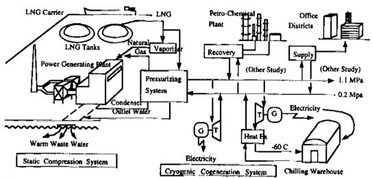
This system is of closed cycle type with hydrogen as working fluid and the capacity of 100kW upto 500kW for both electricity and cold might be a prospective candidate as an independent power unit, since it is an emission-free and simple system.
