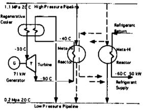
1)System Efficiency: Energy conversion efficiency was evaluated as 38%.
